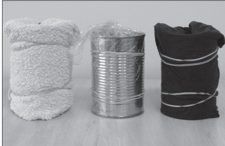
Set up of investigation of ‘Which material keeps things the warmest?’
